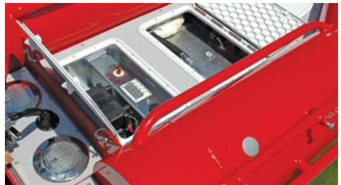
Built-in battery with on/off switch, fuel gauge and electrical switches; built-in fuel tank.
