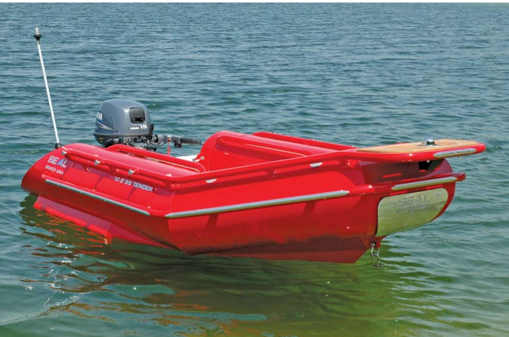
10.0 SS Tender with 15-HP Yamaha, 4-stroke outboard motor.
