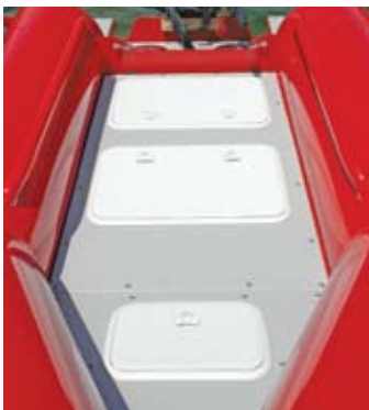
1/2" gray Starboard™ deck and ample below-deck storage.
