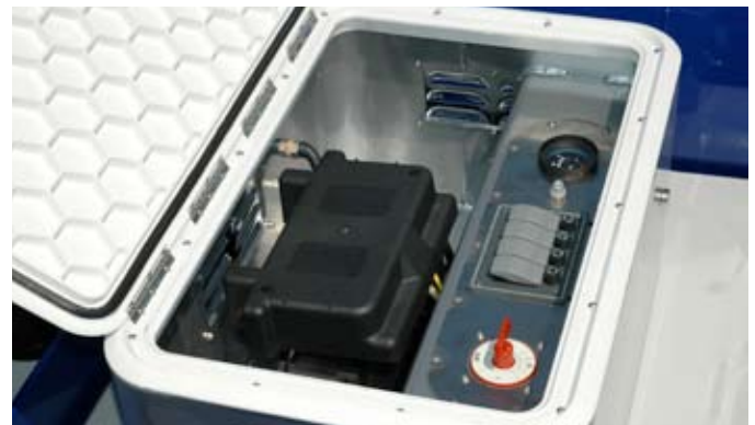
Built-in battery in seat box with on/off switch, fuel gauge and electrical switches.
