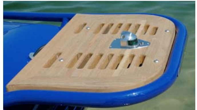
Optional hand-made teak bow pulpit with Accon pop-up stainless steel bow light.
