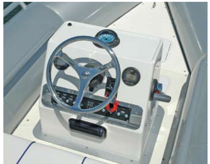
The center console has an 8-switch electric panel with circuit breakers, Teleflex hydraulic tilt steering system and optional stereo and compass.
