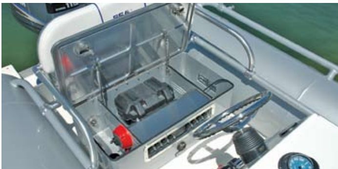
Battery box inside bench seat with on/off switch.
