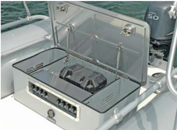
Built-in battery in seat box with on/off switch, fuel gauge and hydraulic lift seat top.
