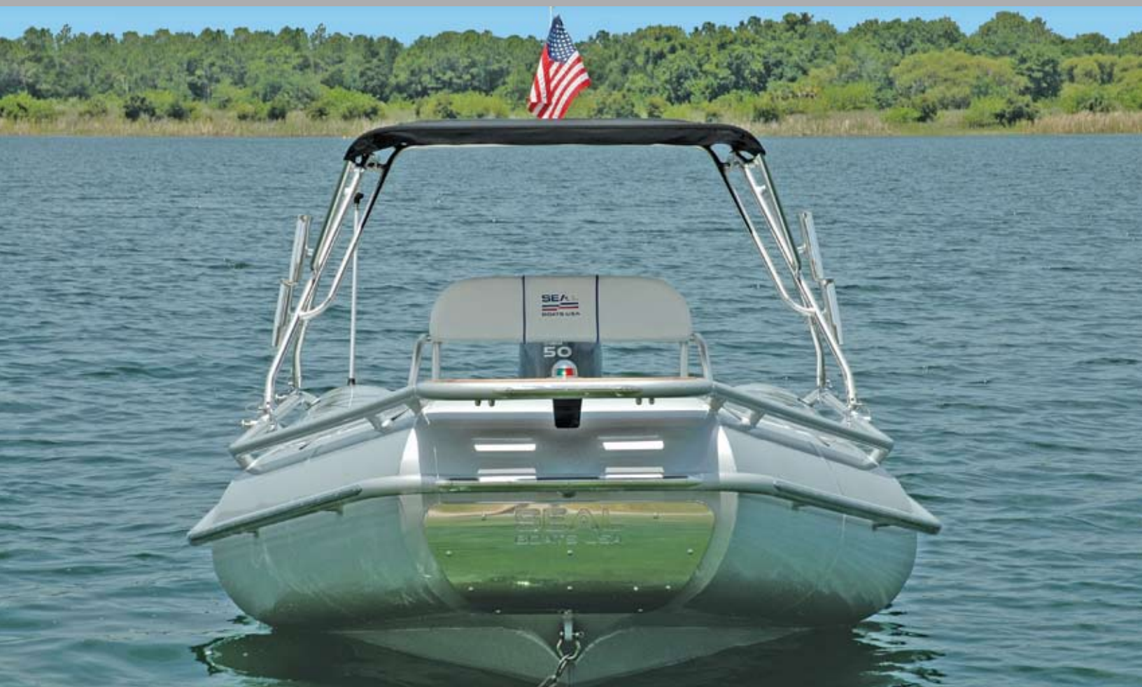
14.5 SS Tender with anodized aluminum powder coating and SEAL™ logo high-polished aluminum chest plate.
